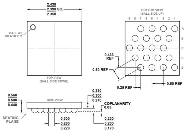
**Figure 48. 20-Ball Wafer Level Chip Scale Package [WLCSP]
