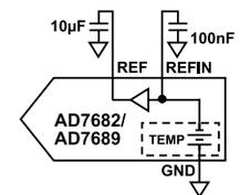
**Figure 33. 2.5 V or 4.096 V Internal Reference Connection**
