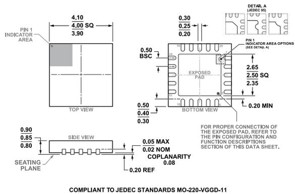
**Figure 47. 20-Lead Lead Frame Chip Scale Package [LFCSP]
