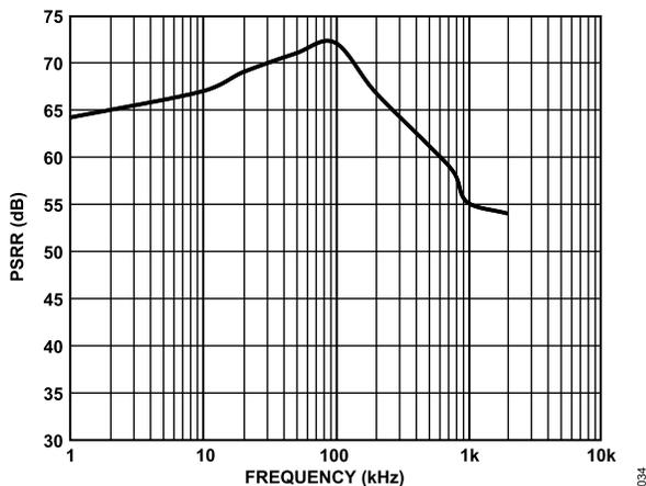
Figure 36. Power Supply Rejection Ratio (PSRR) vs. Frequency
