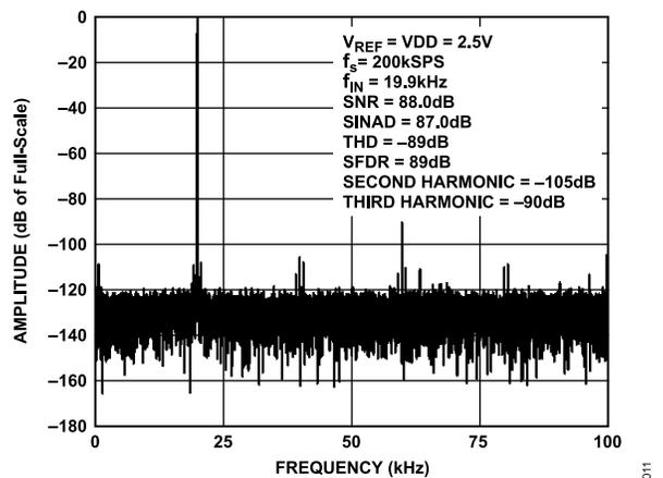
Figure 13. 20 kHz FFT, VREF = VDD = 2.5 V
