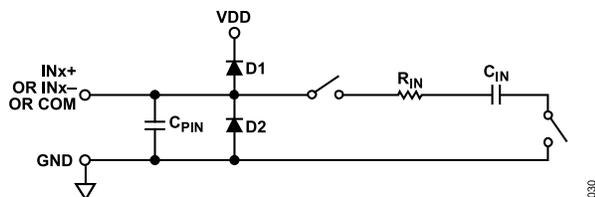
Figure 30. Equivalent Analog Input Circuit
