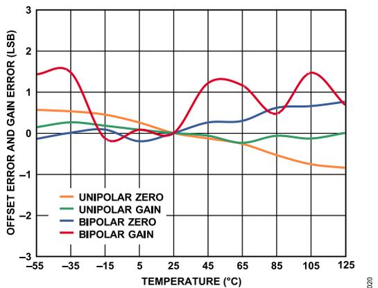
Figure 22. Offset and Gain Error vs. Temperature
