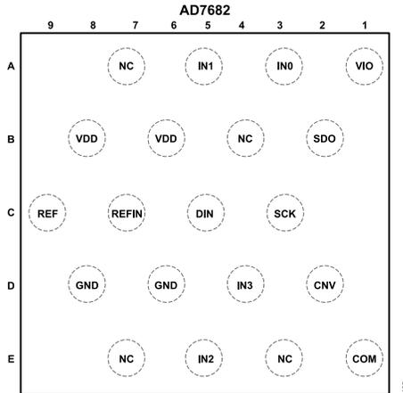
Figure 6. AD7682 WLCSP Pin Configuration
