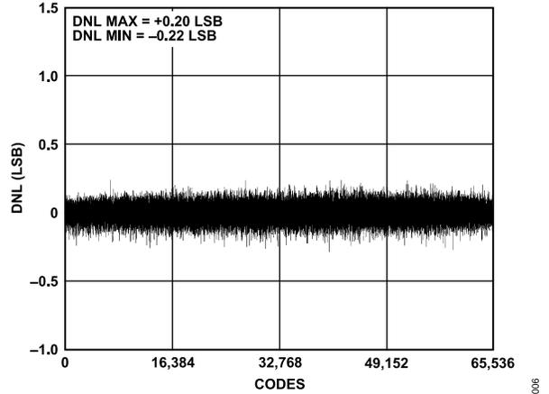
Figure 11. Differential Nonlinearity vs. Code, VREF = VDD = 5 V
