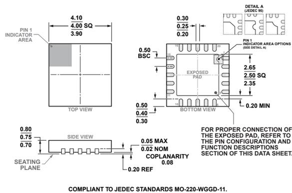
**Figure 46. 20-Lead Lead Frame Chip Scale Package [LFCSP]
